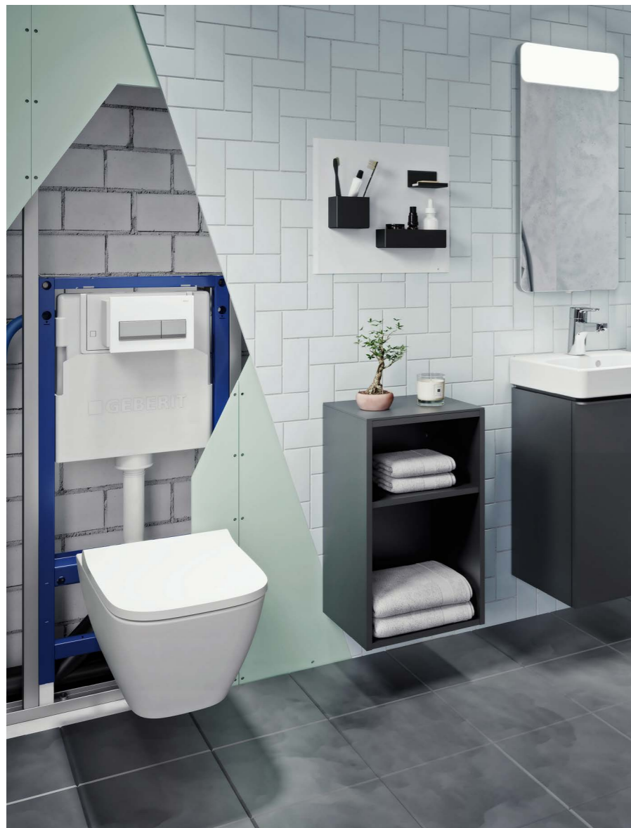
TWO CISTERN HEIGHTS The Geberit Alpha concealed cistern can be installed at a height of 82 cm and 112 cm. All the Alpha cisterns come with a water-saving dual flush system.
