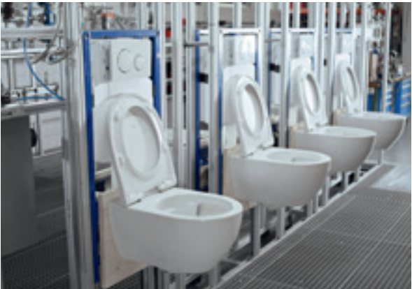
↑ CERAMIC CHECK Geberit ceramics undergo strict quality controls after production before they are sent to our customers.
