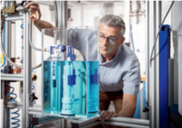
↑ HYDRAULICS EXPERTISE Geberit's sanitary technology laboratories put flush and fill valves through their paces to demonstrate maximum hydraulic performance and pass long-term durability tests.
