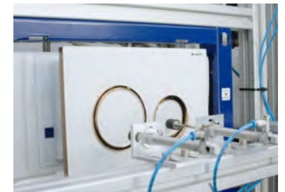
↑ PRESSURE TEST The components for flush actuation must be able to withstand at least 200,000 actuations, corresponding to a service life of around 50 years.
