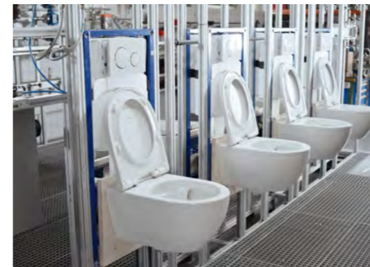
↑ CERAMIC CHECK Geberit ceramics undergo strict quality controls after production before they are sent to our customers.
