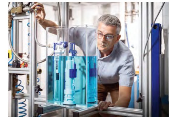
↑ HYDRAULICS EXPERTISE Geberit's sanitary technology laboratories put flush and fill valves through their paces to demonstrate maximum hydraulic performance and pass long-term durability tests.
