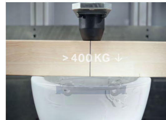
↑ LOAD TESTS Geberit ceramics must pass stringent load tests and reliably fulfill all relevant standards.
