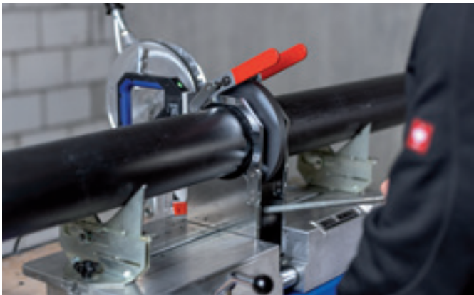
GEBERIT WELDING MACHINES Geberit Universal and Media welding machines are easy to operate and quick to retrofit. Thanks to their particular robustness, they are well suited to both prefabrication in the repair shop and use at the building site.
